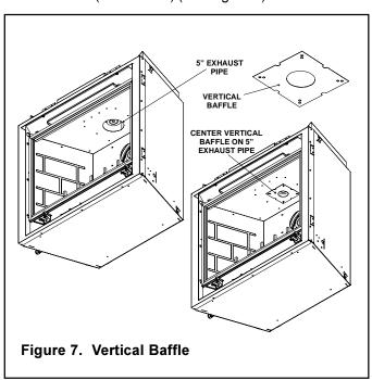
**NOTE:** Center the vertical baffle over the 5" exhaust pipe. Fasten in place with self tapping screws.
